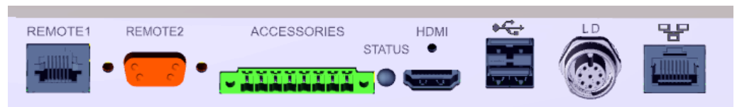
Fig. 4: Connections for accessories and control signals at the back side of the device.
